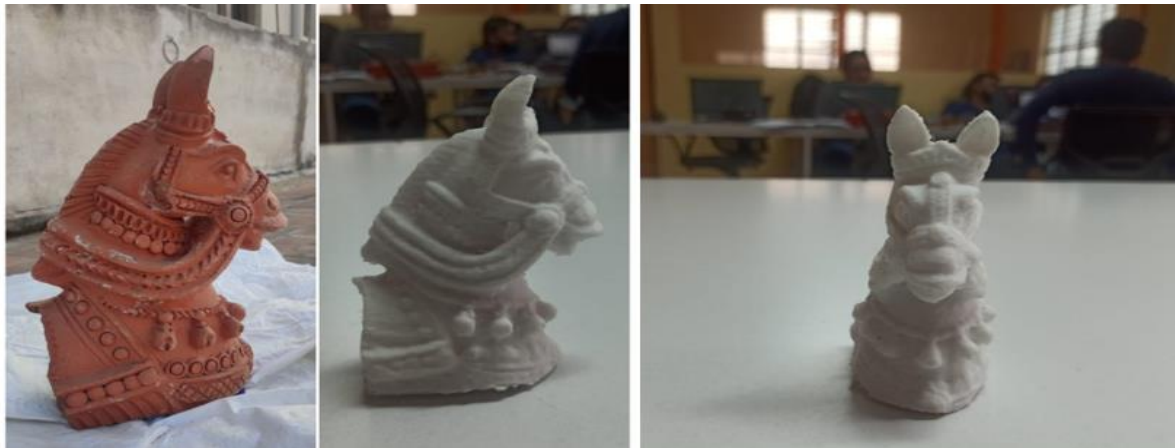
Figure 17: Comparison of Real object and 3D printed object
