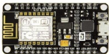
Figure 16 The LED On-board of ESP8266
